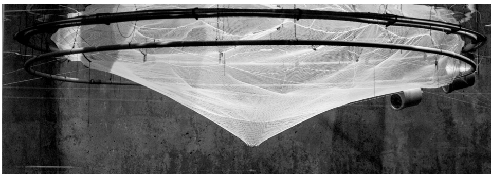
Fig. 2. The model of the Polarcircle type cage with the sinker tube in position for delousing.
